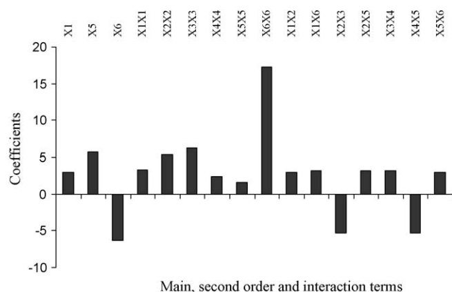
Fig. 5. Significant main, second order and interaction terms for decolorization and COD reduction of reactive azo dye rifacion yellow HE4R by using combined ultrasound/activated carbon.
